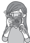
Do not cover the flash sensor or AE light sensor with your finger while taking a photo.
